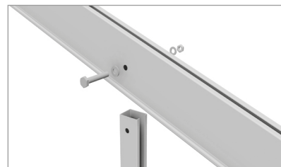
Connection detail leg - rafter
